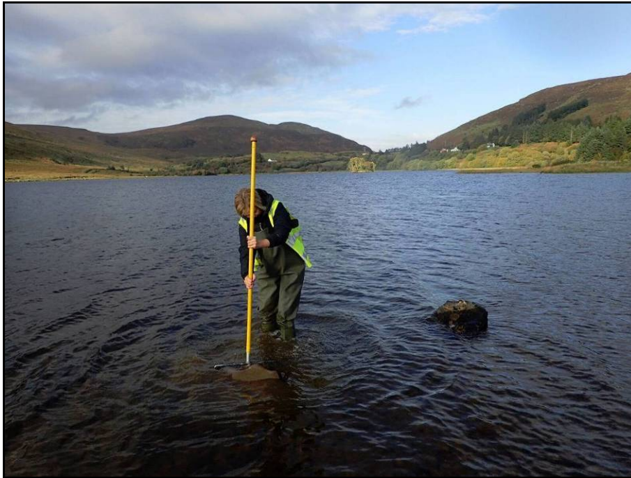
Plate 7 Kick sampling using a dip net was used to sample macroinvertebrates along the littoral margins of the lake.
