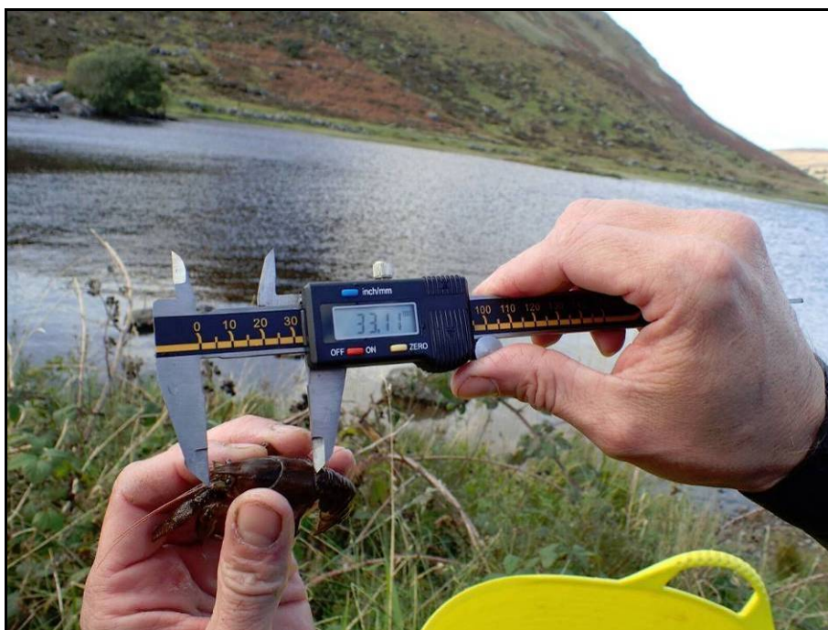
Plate 9 Crayfish carapace length measurement using digital Vernier calipers.
